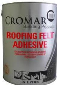
A solvent based high viscosity bituminous adhesive with strong initial "grab" properties. Felt Adhesive is a cold applied roofing adhesive formulated for convenience and safety, ensuring affinity and a strong, final bond to roofing felts. It is used for bonding all types of roofing felts to metal, timber or concrete, sealing roofing felt laps and bonding chippings to flat roofs. Felt Adhesive is applied at 2 square metres per litre.
